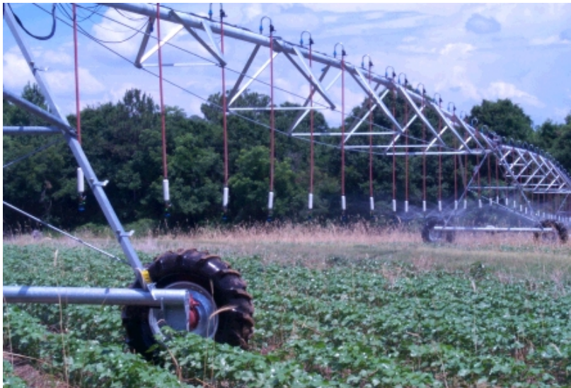
Variable Rate Irrigation (VRI) is one means to conserve water by applying to prescribed areas (Photo by Calvin Perry, 2004)
